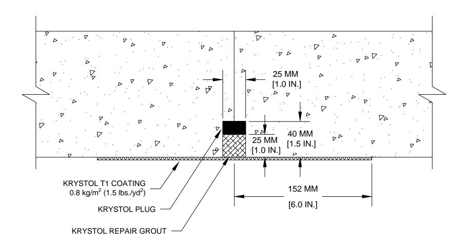
LEAK OR JOINT REPAIR - WALL TO WALL
